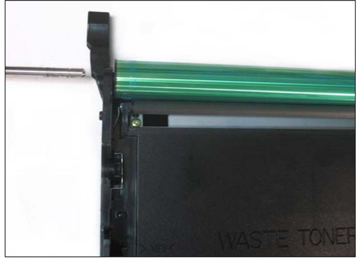
25. Follow through until the axle is completely removed.
