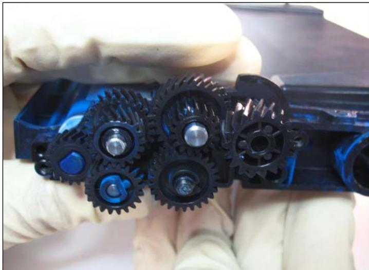
**REMOVING THE GEARS**
