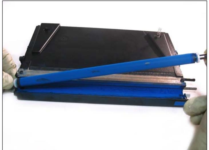
19. Remove the developer roller as shown.
