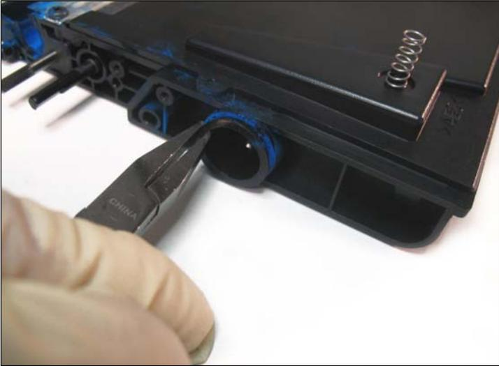
20. Locate the fill plug on the gear-side of the cartridge. Using a pair of pliers, carefully pull it out.
