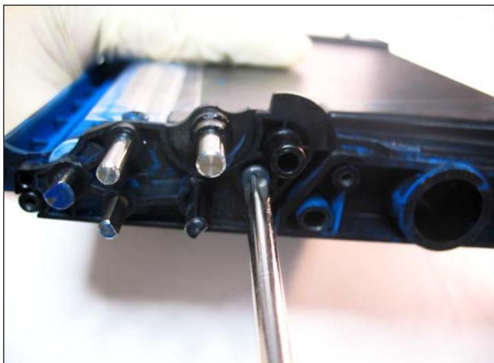
**GEAR-SIDE SUPPORT PLATE REMOVAL**
