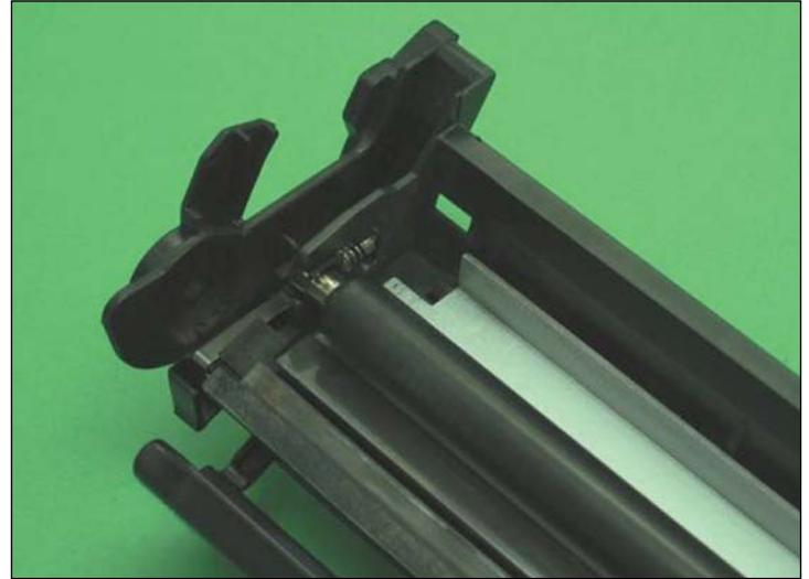
2. Install the PCR as shown. If you are using an OEM PCR, please make sure it is carefully cleaned.
