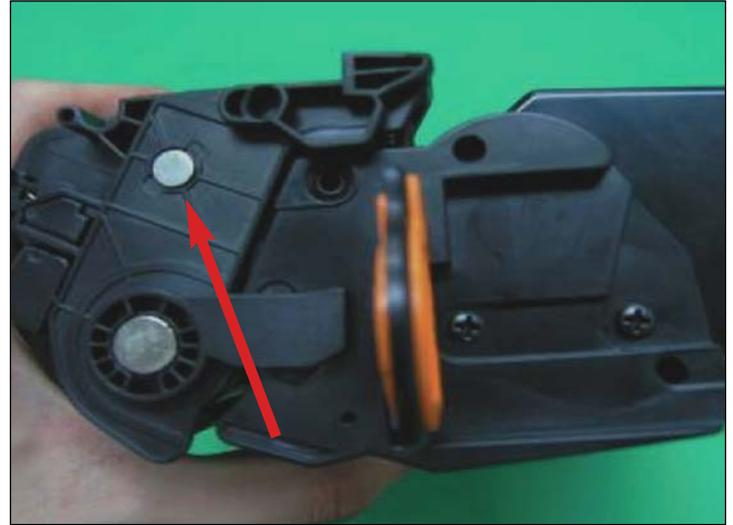
17. Assemble the Hopper side and Waste Hopper together and insert the hinge pin on each side to hold them together.
