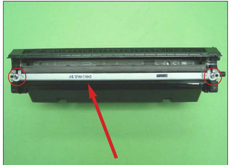
11. Install the doctor blade into the Hopper, and place the Mag Roller wiper on each end of the Doctor Blade. Tighten the two screws (shown) that hold the doctor blade and wipers in place.
