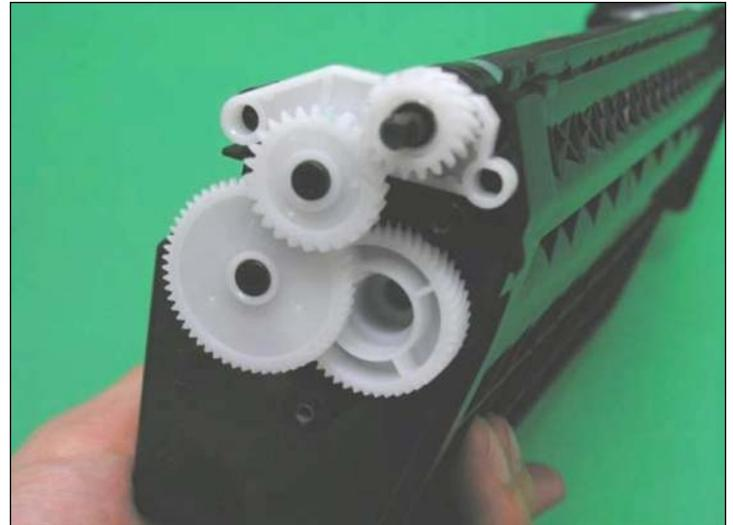
15. Install the Mag Roller as shown in the Hoper as shown in the photo. Then insert the Right Stabilizer, and all drive gears on the right side of the hopper.
