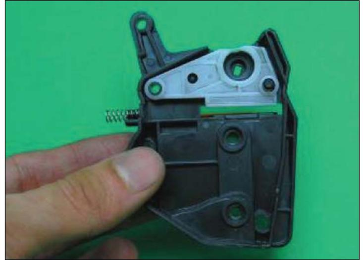
13. Install the Left Stabilizer on the P2015 Left End Cap as shown.
