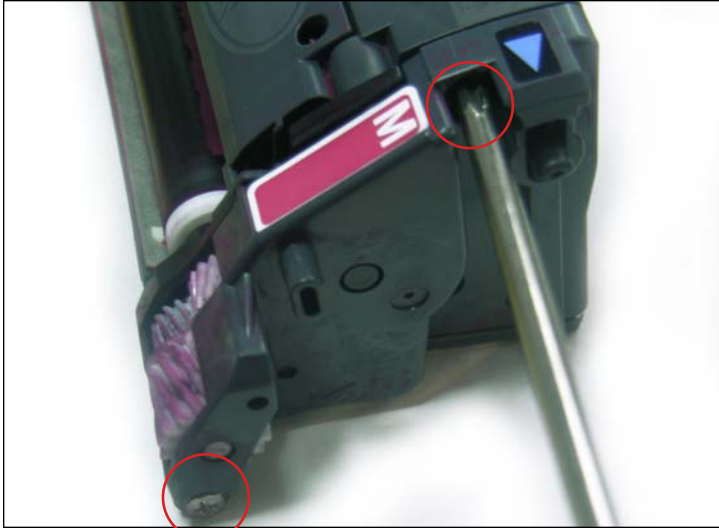
3. Remove the two screws on the opposite side (with gears) that hold the end cap in place.
