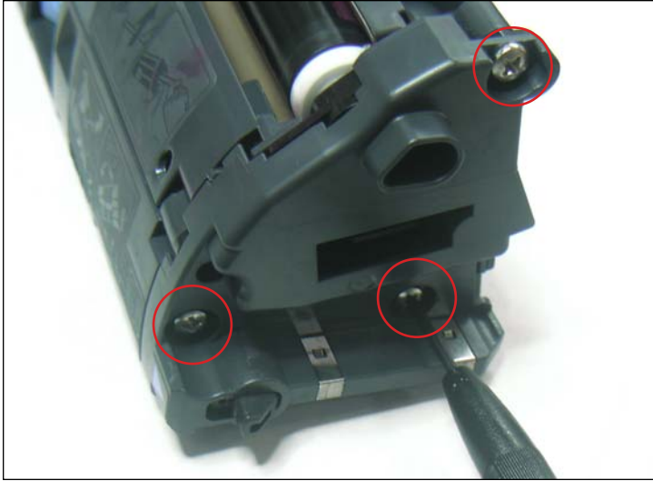
1. Remove the three screws that hold the end cap (gearless side) in place as shown (note that one screw will be smaller than the other two).
