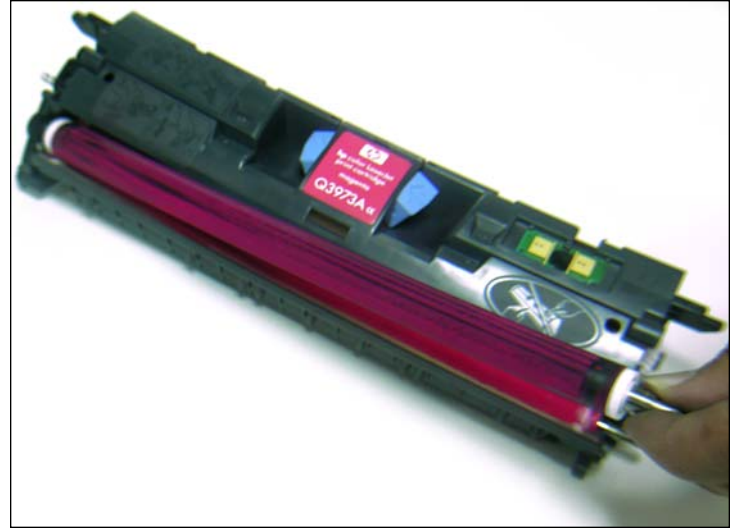
10. Remove the developer roller as shown.
