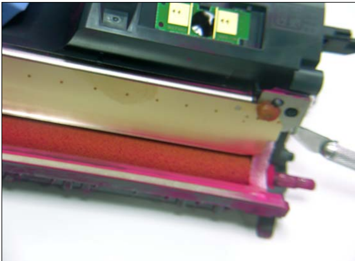
15. Third, using an x-acto knife carefully cut away the adhesive gum that seals the back ends of the doctor blade and the plastic cartridge.
