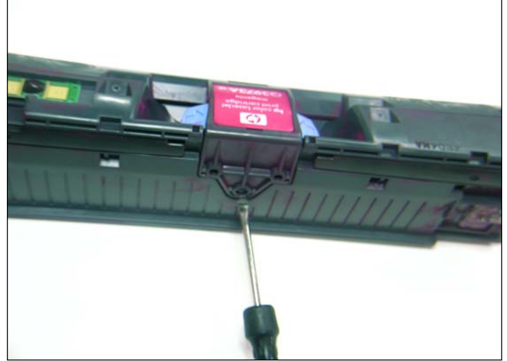
12 First, use a small flathead screwdriver to pry off the back of the doctor blade cover as shown.
