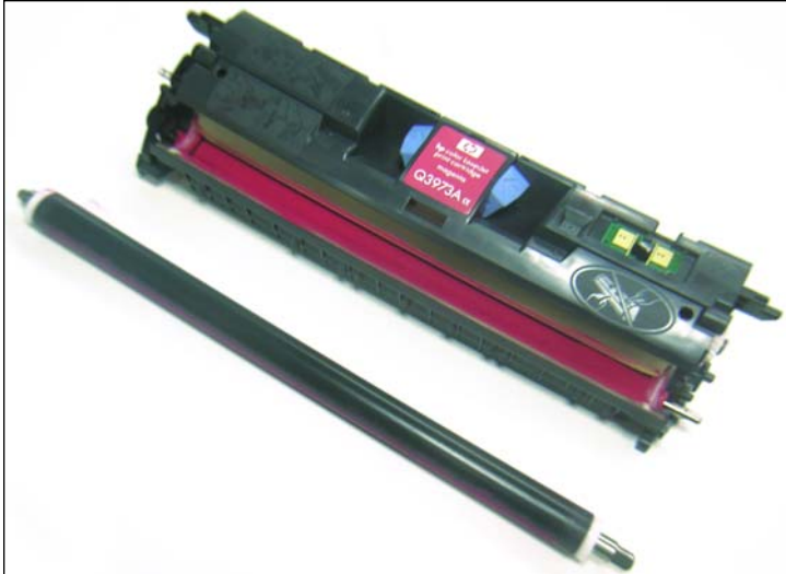
11. Do not lose the white bearings located at the ends of the developer roller.
